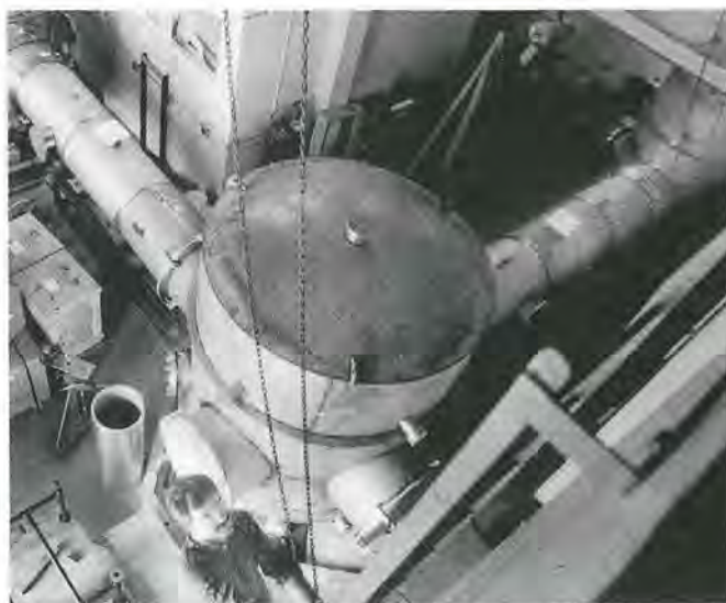
Detecting gravity waves. Researcher checks the vacuum enclosure for MIT's gravitational wave interferometer. This L-shaped gravity wave sensor is a precursor of the highly sensitive full-scale laser interferometer detector proposed by MIT and Caltech physicists. Such devices detect the gravity waves generated by the sudden acceleration of mass.
