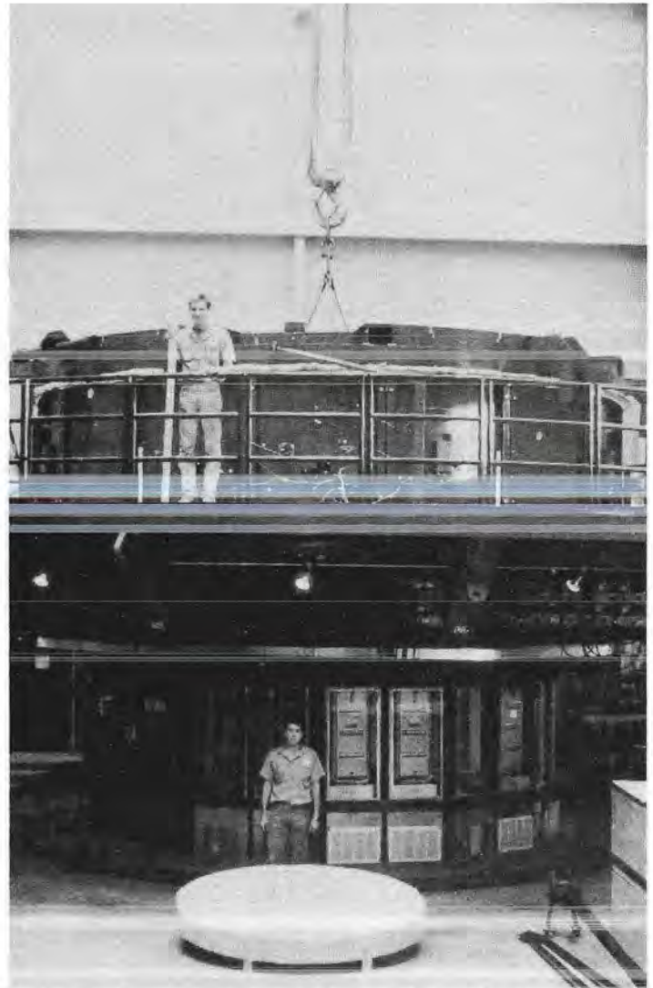
Innovative design. Special rotating furnace designed by University of Arizona's Roger Angel creates the rough parabolic curve in telescope mirrors that ordinarily takes months of polishing to achieve.
