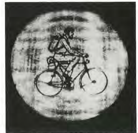
Novelty filter. Dana Anderson and Jack Feinberg collaborated on an ingenious new optical circuit that memorizes the shape and position of an object. A three-dimensional image of the object forms in the optical circuit—known as a “Novelty Filter”—but the image quickly fades unless the object moves or the background scenery changes, as seen in these two photos.
