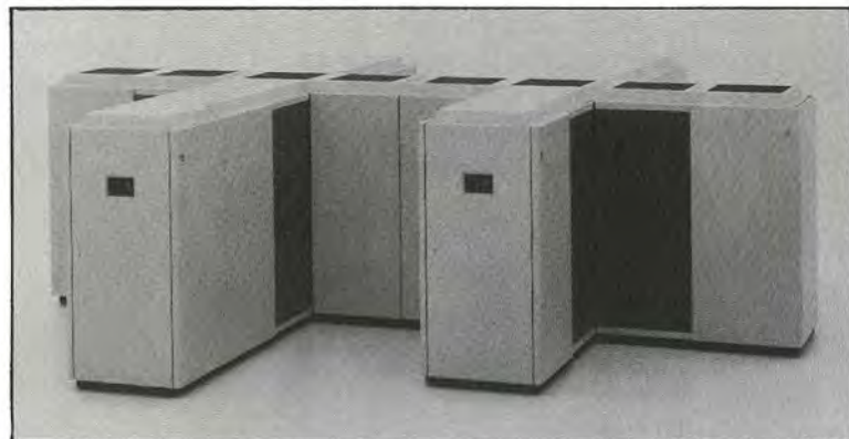
Most powerful mainframe. The IBM 3090 Model 600E supercomputer, recently installed at Cornell University, provides up to 60 percent more computing power than IBM's largest previous model.
