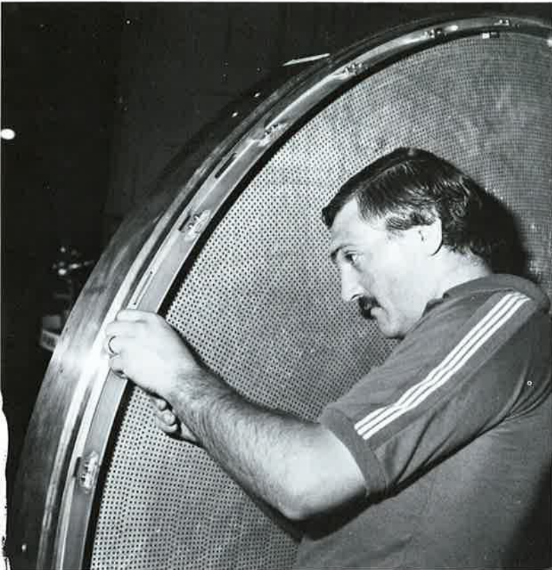
Detector Construction. A researcher at the Cornell Electron Storage Ring (CESR) assembles the large central drift chamber. It tracks charged particles in an experiment designed to study the basic structure of matter.
