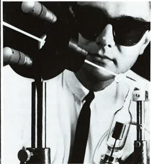
Laser progress. This is one of the first argon ion lasers. (Photo courtesy of Hughes Aircraft Company)
