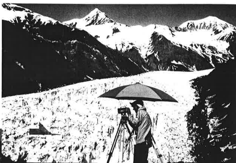
Alaska's Variegated Glacier. Photo at bottom left shows the lower middle part of the glacier before that section began to surge. Picture at top left is the same view a year later, during the surge. In third shot, scientist measures the glacier motion with an electronic distance meter, using a laser beam.
