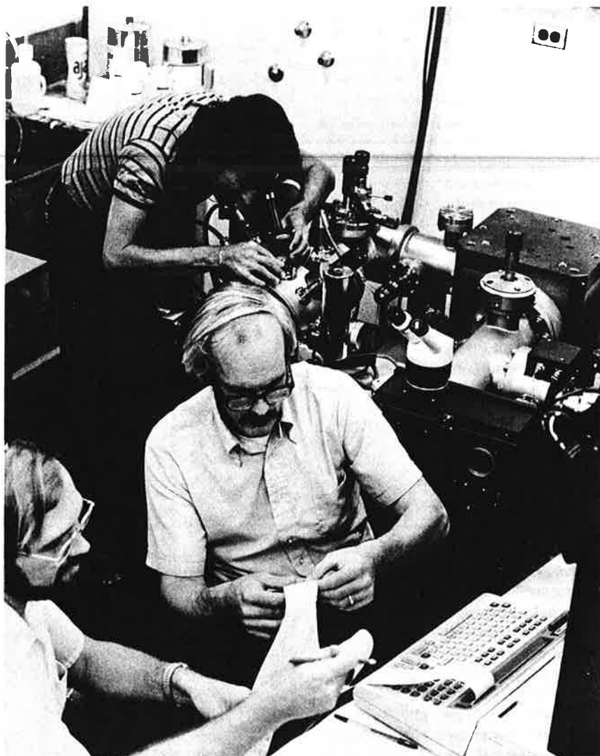
Sophisticated tools. Researchers use an ion microprobe at the Massachusetts Institute of Technology for trace-element and isotopic analyses on minute parts of rocks. Such studies enable earth scientists to understand the deep-earth conditions under which rocks form.
