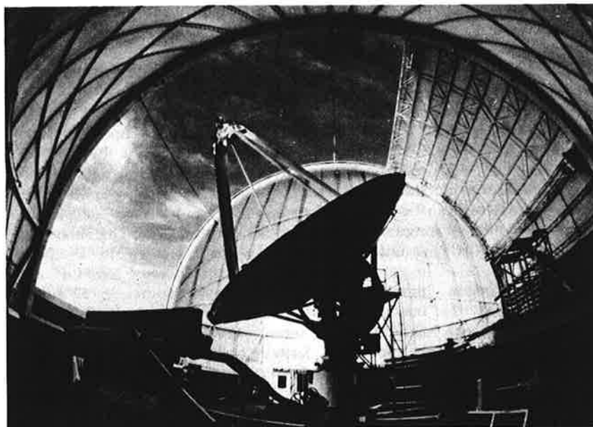
Interstellar organics. The National Radio Astronomy Observatory's 36-foot millimeter-wave telescope at Kitt Peak, a key instrument in the discoveries of organic molecules in space, will be an even more effective tool as a result of equipment upgrading during the past year.
