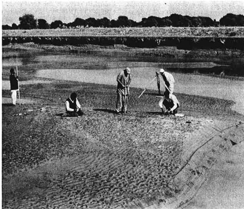
Water research. As part of a U.S.-Pakistan joint research project, scientists (left) meter the water surface level of a Link Canal and take a soil core (right) to determine particle size of bottom sediments. The Link Canals, built to redistribute scarce water among Pakistan's rivers, are part of one of the world's most ambitious water development projects. Their size and variety make them valuable for research on the design of modern irrigation channels. (Photos by Kahlid Mahmood/George Washington University.)
