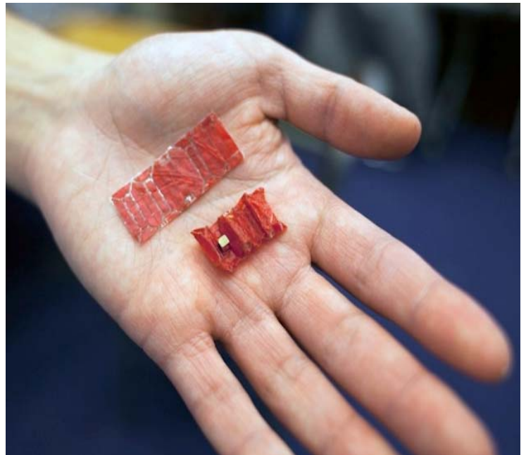
NSF-funded researchers have developed an origami robot that folds into an ingestible capsule. Credit: Melanie Gonick, MIT
