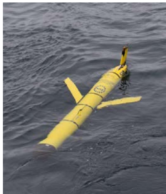
All Global and Coastal Arrays utilize gliders to collect physical and biogeochemical data to supplement those collected by the stationary moorings. At the Global Arrays, the gliders collect data from the subsurface moorings using acoustic technics and relay the data to shore via satellite. Credit: Sawyer Newman, WHOI.
